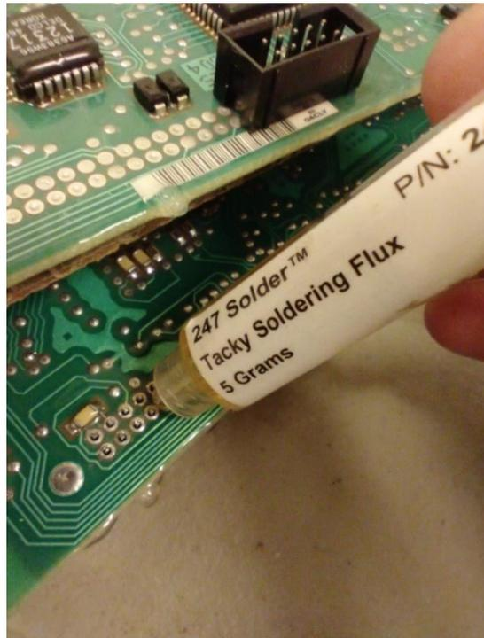
Also in this picture above you can see the headers orientation. The opening is facing away from the pcb edge and toward the pcm wiring connectors. This is the same for both T & E sides. If you get it backwards, pcm **DAMAGE WILL OCCUR** once you attempt to use the LT-UNBRICK tool and RESET Tab that is included in this
